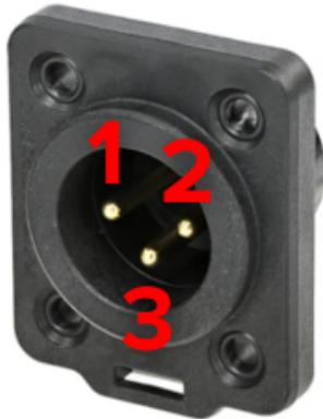
The XLR male chassis, pin 1 is the grounding, 2 and 3 are the dry contact pins.
